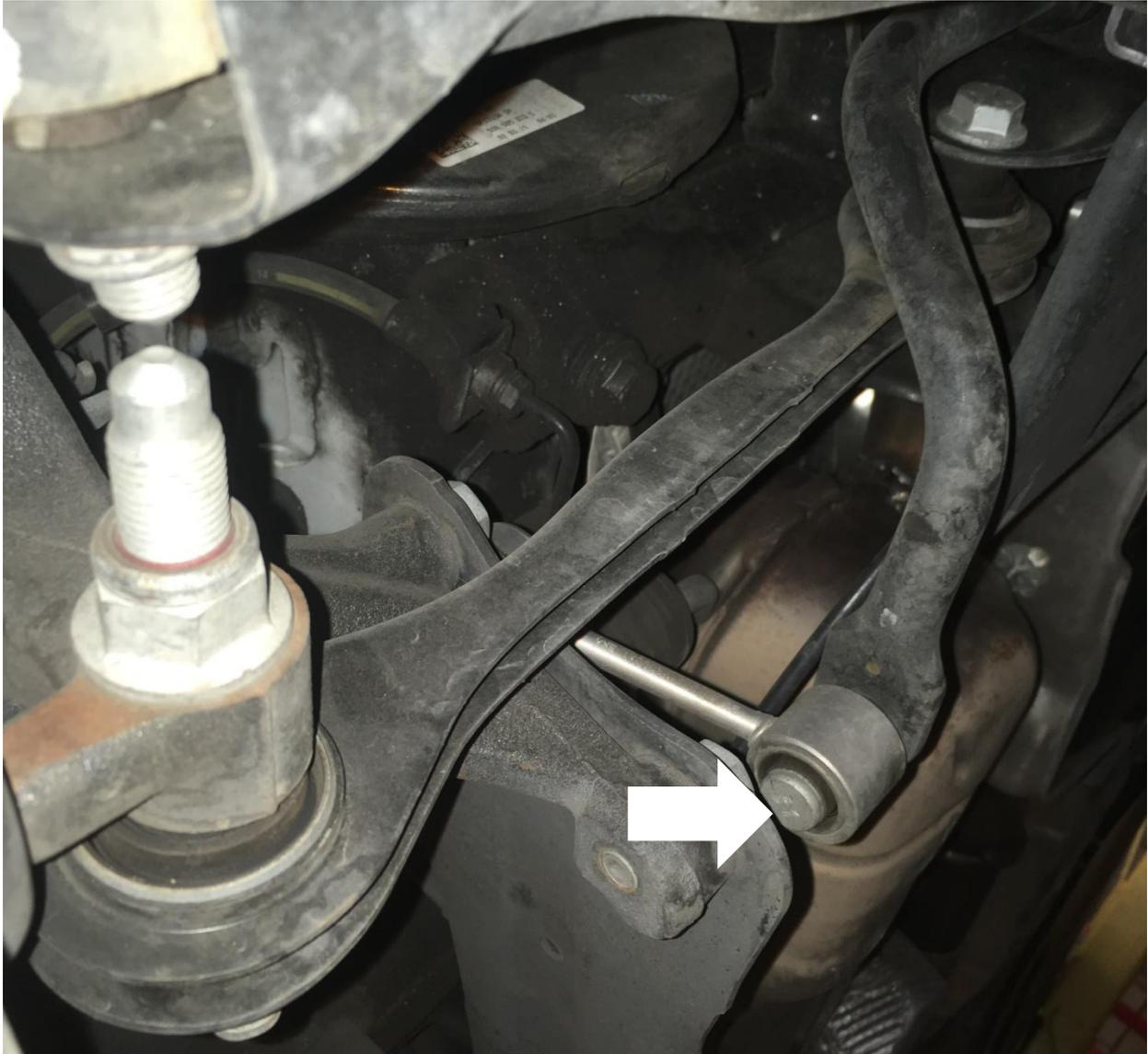
**Step 6:** Remove the bolts from the sway bar brackets for sway bar removal. T50 inverted Torx bit is required for removal.
